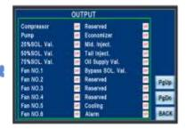
OFF means the point have no signal input, ON means the components are working normally.
